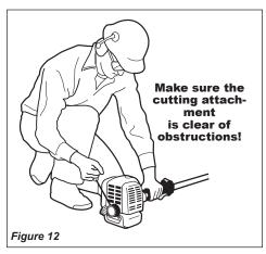
5. While holding the outer tube firmly with left hand. Use your other hand to slowly pull the recoil starter handle until resistance is felt, then pull quickly to start the engine.
